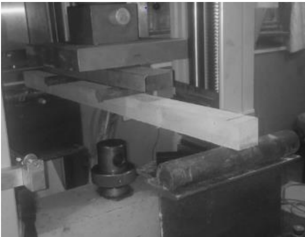
Figure 2: Four Point Bending test Setup
