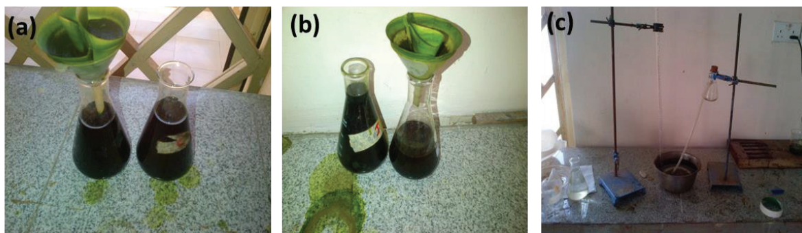
Fig. 1: (a) Filtration of Cascabela thevetia extract, (b) Filtration of Jatropha curcas extract, (c) Apparatus setup for gasometric analysis
