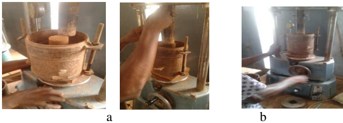
Figure 4: (a) Process of loading the mould for compressive strength tests and (b) California bearing ratio compressive strength testing machine
