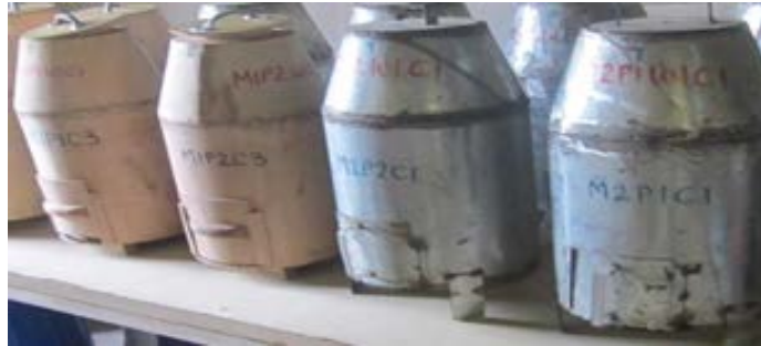
Figure 1. Wooden and Galvanised mild steel(GMS) storage structures
