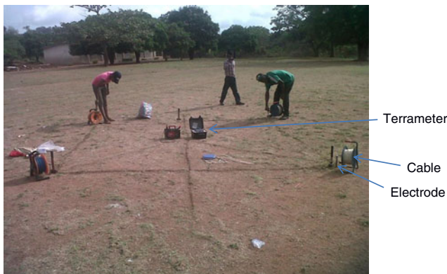
Fig. 5 Field arrangement of the cross-square array
