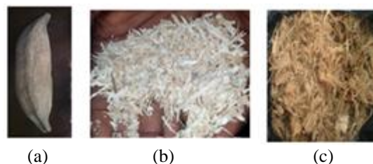
Figure 1 Materials used before processing: (a) Kapok pod; (b) Sugarcane bagasse; and (c) Coconut fibre (coir)
